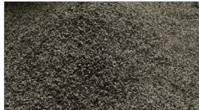
Scrap reground to be used in DaVinci composite roofing tiles:
